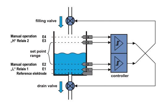
In liquid reservoir, four electrodes (E1..E4) are mounted in the medium, at heights corresponding to the required switching point. According to water contact, the fill level is indicated through 4 green LED's L1 to L4. If the reservoir is completely empty, the red LED glows.
